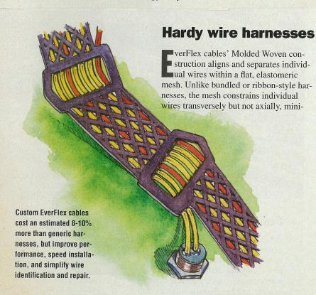
mizing wire tension during bending. Custom designed, they bend at prescribed points and snake around obstacles to protect wires from chafing or pinching during machine assembly or repair.
