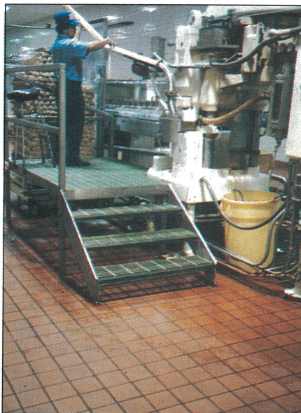
Glassfibre stair treads (Chemtred) combine with walkways to provide both sanitation and safety. Similar pedestals and supports expedite clean-in-place sanitation procedures. The stairs and walkways will not rust, corrode or ever need painting
